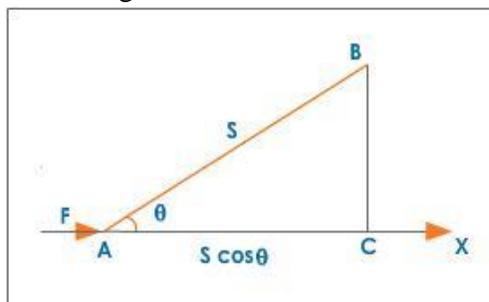
Displacement in the direction of the force = Component of  $S$  along  $AX$
