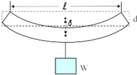
A bar of length  $l$ , breadth  $b$ , and depth  $d$  when loaded at the centre by a load  $W$  sags by an amount given by  $\delta = \frac{W l^3}{4bd^3Y}$
