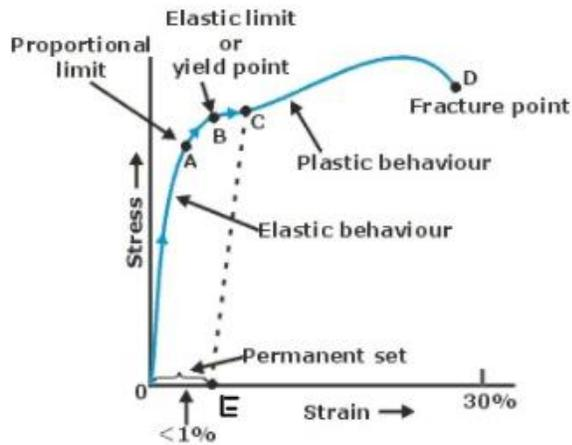
Figure shows the stress-strain curve for a metal wire which is gradually being loaded.
