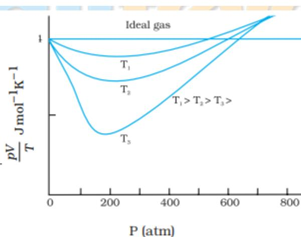
*Real gases approach ideal gas behaviour at low pressures and high temperatures.*
