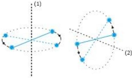
There are two independent axes of rotation (1) and (2) normal to the axis joining the two oxygen molecules. It has 3 translational and 2 rotational degrees of freedom
