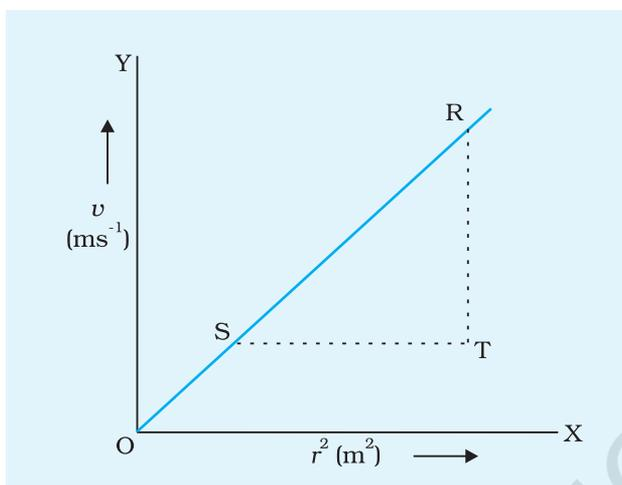
The relation given by Eq. (E 13.3) holds good if the liquid through which the spherical body falls freely is in a cylindrical vessel of radius  $R \gg r$  and the height of the cylinder is sufficient enough to let the ball attain terminal velocity. At the same time the ball should not come in contact with the walls of the vessel.
